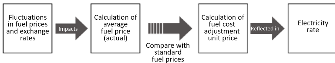
Figure 1: Image of the calculation flow for the fuel cost adjustment system
